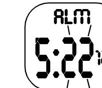
Press or hold down ADV./ST./SPL. to advance through the digits, then press MODE. The minute digits flash.
